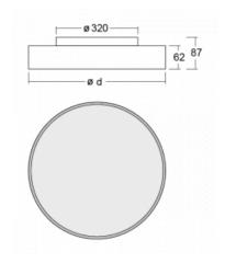
Luminaire power80.7 Winput\*ON/OFFConnection of the<br/>luminairesON/OFFElectrical voltage220-240VFrequency50/60Hz
