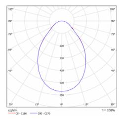
Luminaire power 94.8 W input\* Connection of the ON/OFF multiwatt luminaires Electrical voltage 220-240V Frequency 50/60Hz
