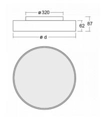
Luminaire power<br/>input\*54.5 WConnection of the<br/>luminairesDALIElectrical voltage220-240VFrequency50/60Hz
