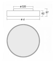
Luminaire power<br/>input\*40.3 WConnection of the<br/>luminairesDALIElectrical voltage220-240VFrequency50/60Hz
