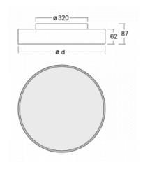
Luminaire power<br/>input\*45.5 WConnection of the<br/>luminairesDALIElectrical voltage220-240VFrequency50/60Hz
